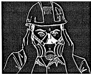
Negative Pressure Fit Test Cover inlets and try to inhale
