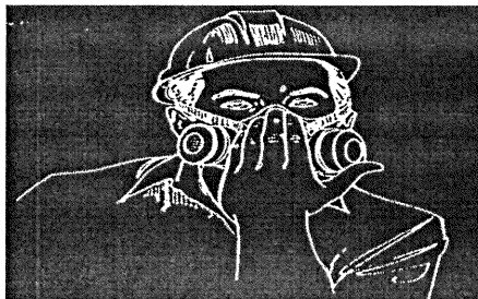
Positive Pressure Fit Test Cover exhalation valve and try to exhale
